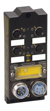
The FDNQ-4AI-V/I-T station has four analog input connectors. Each connector provides a connection point for an analog transducer. The transducer can be selfpowered or loop powered. This station has a 16-bit resolution for the analog signal. Preset current and/or voltage modes are 0 to 10 V, -10 to +10 V, 0 to 20 mA and 4 to 20 mA.
